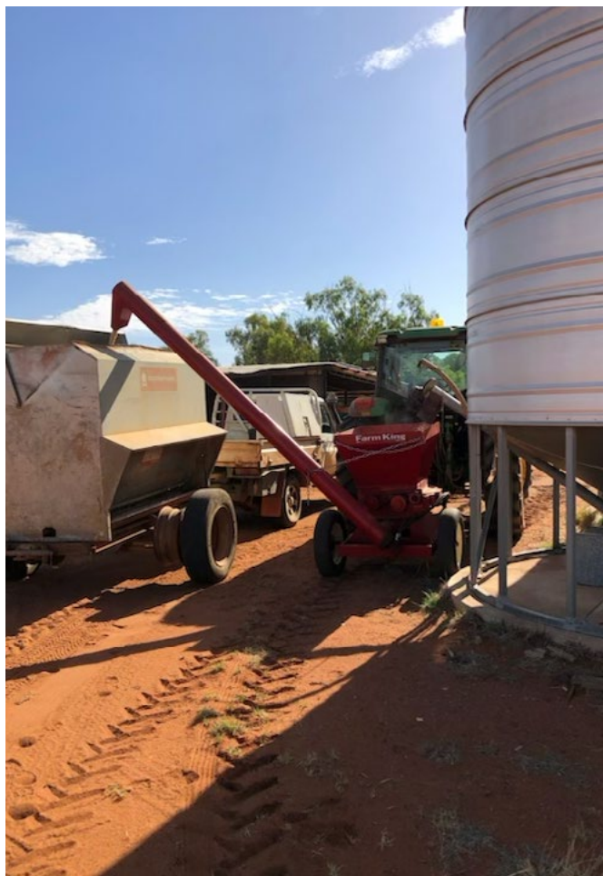
Image 7 The lupin milling and loading process occurs in one production line, from silo (right), to roller mill (center) and finally directly into the mobile feeder (left), which is then carted out to the demonstration paddock
