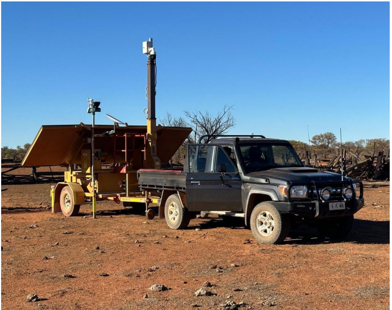
Image 8 Automated portable monitoring system at Challa Station
