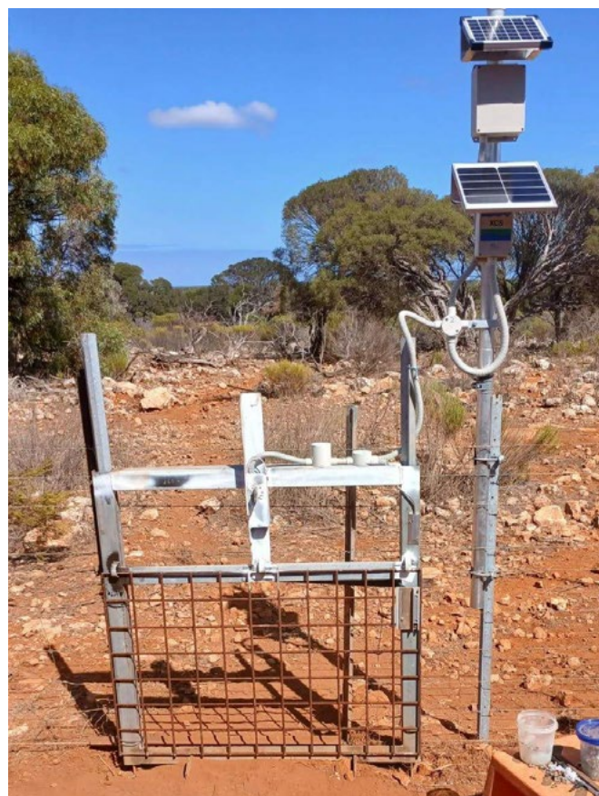
Image 11 Automatic gate that can be triggered shut using a mobile phone
